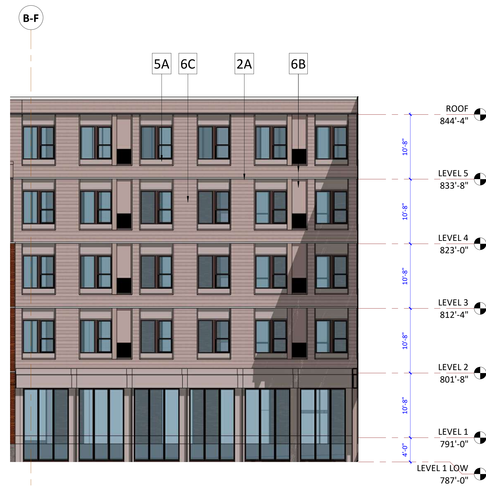
4 BUILDING B - COURTYARD ELEVATION - WEST A3.2E 1/8" = 1'-0"
