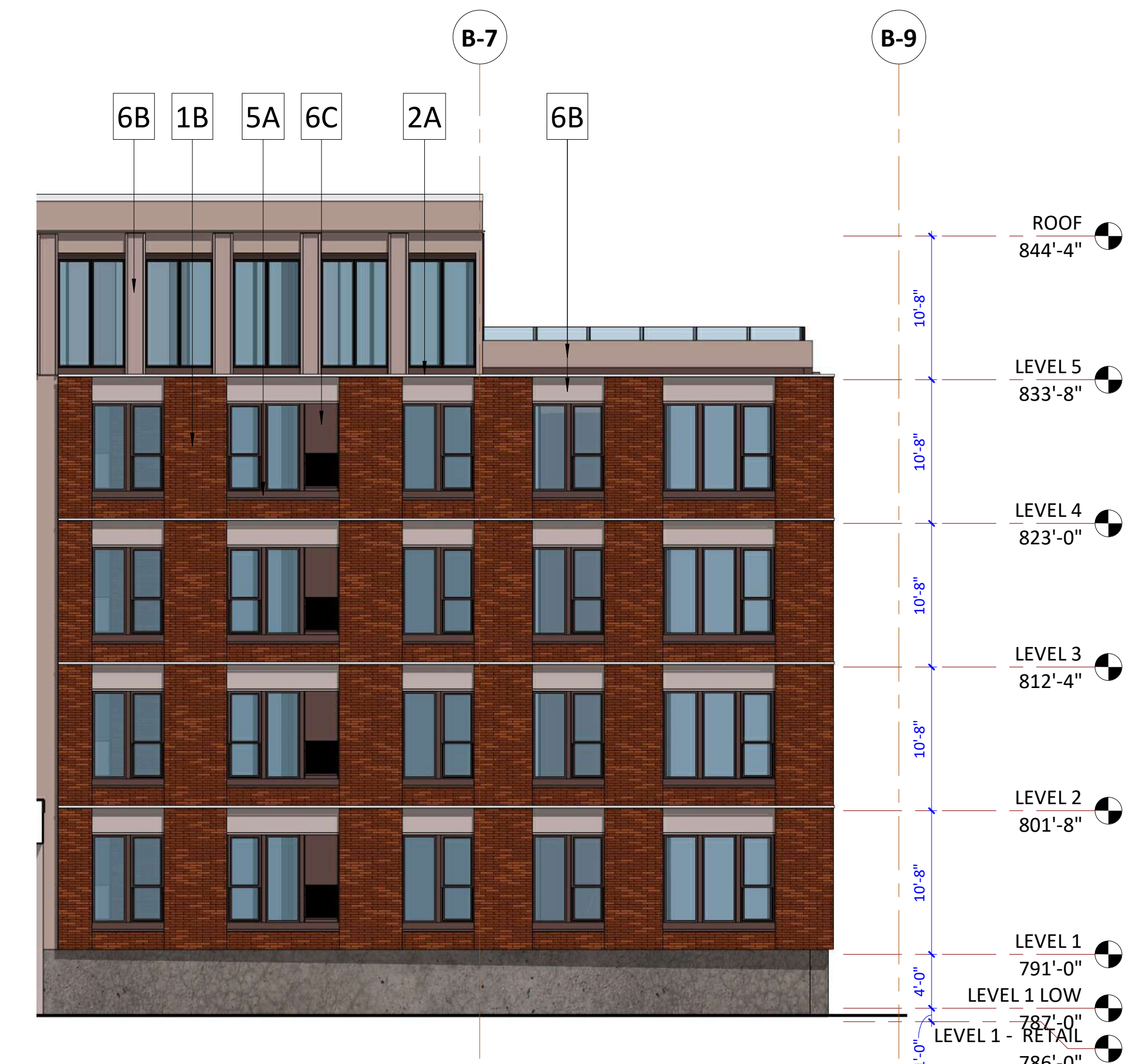
1 BUILDING B - COURTYARD ELEVATION - NORTH A3.2E 1/8" = 1'-0"
