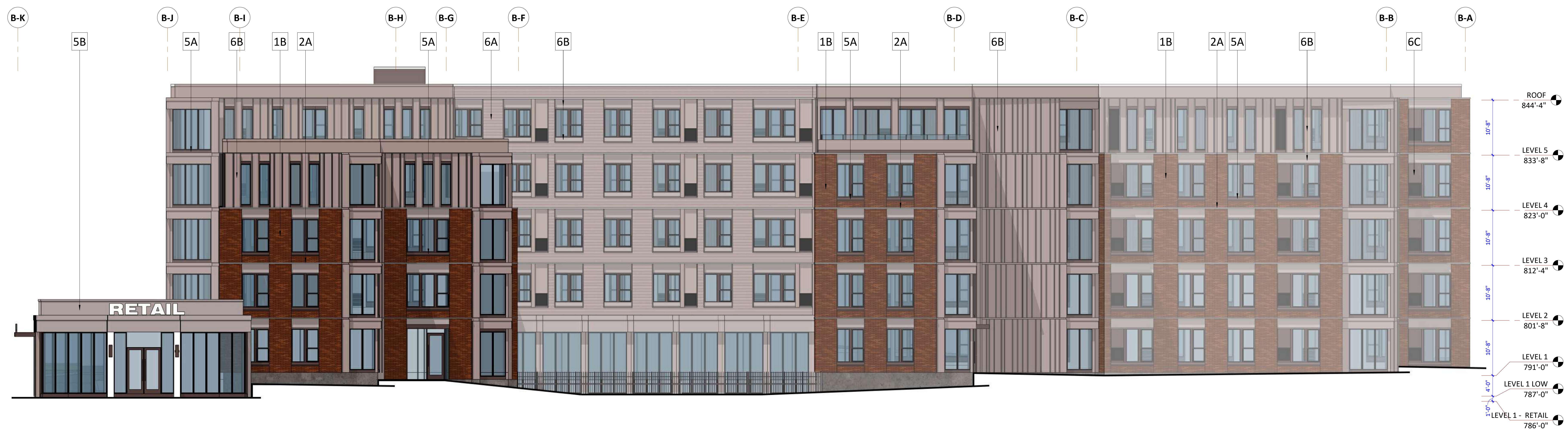
1 BUILDING B - EAST ELEVATION A3.2C 3/8" = 1'-0"
